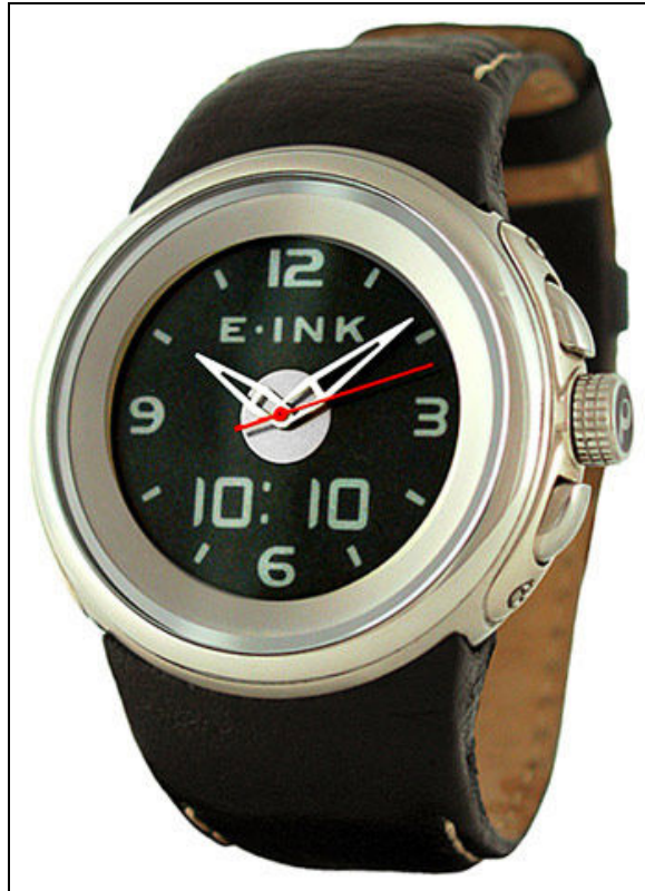
Phosphor watch utilizes E Ink display to enable customizable watch dials
